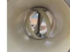
Image 15: Energy recovery from flow in a pipe. (Source: DMU, 2015)
